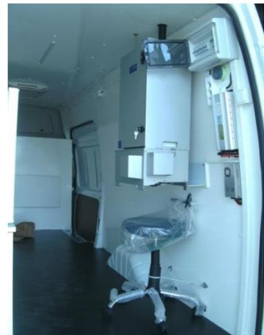
Both stations are configured to measure gaseous and aerosol air pollutants including nitrogen dioxide (NO<sub>2</sub>), oxides of nitrogen (NO<sub>x</sub>), carbon monoxide (CO), and particulate matter fractions of PM<sub>1</sub>, PM<sub>2.5</sub>, PM<sub>10</sub> and total suspended particulates (TSP).
